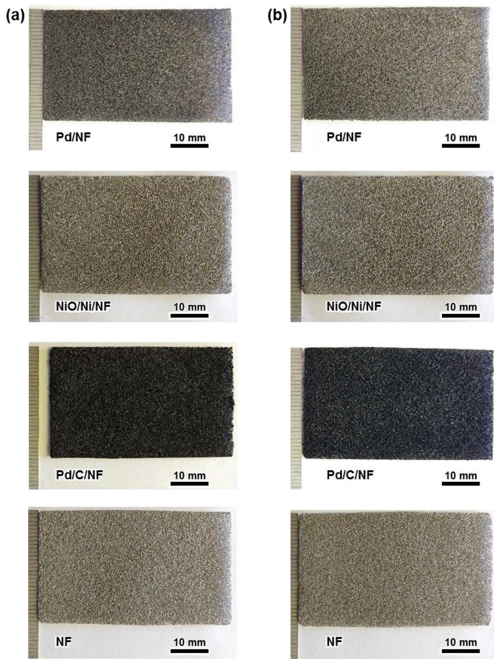
Figure S1. Digital photos of large electrodes (a) before and (b) after electrooxidation tests.
